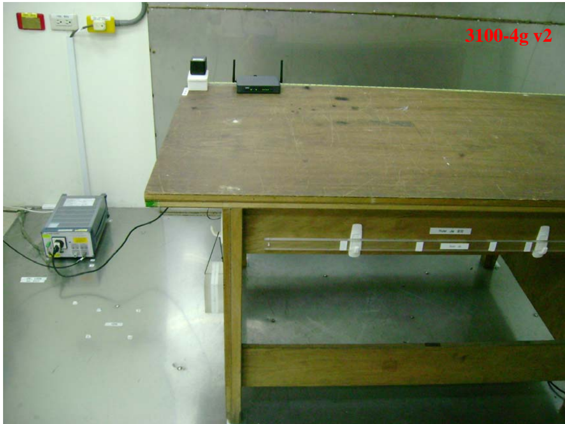
Photo 1: Conducted Emission Test Set-up photo
