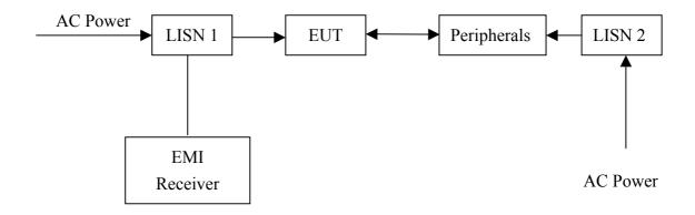
The EUT are connected to the main power through a line impedance stabilization network (LISN). This provides a 50 ohm/50uH coupling impedance for the measuring equipment. The peripheral devices are also connected to the main power through a LISN that provides a 50ohm/50uH coupling impedance with 50ohm termination.
