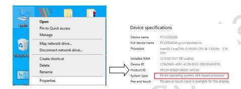
The OS type MTK strongly recommends use Windows10 64-bit operating system. Users should set Windows10 64-bit OS under test mode according to following steps:
