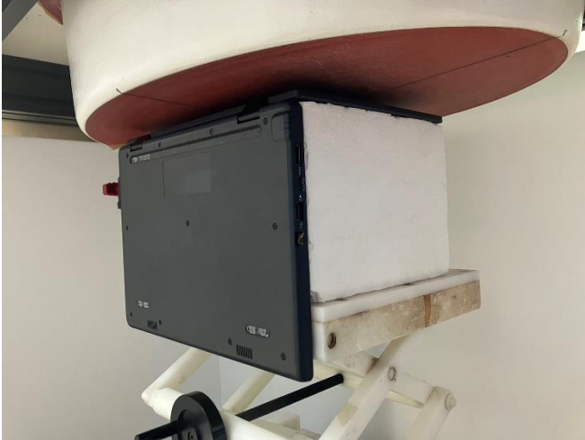
Testing Setup for Body, Back of Display Screen at 25 mm
