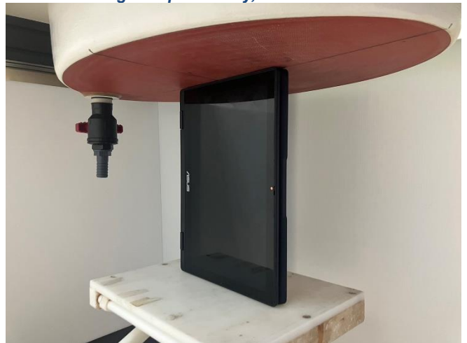
Testing Setup for Body, Left Side at 0 mm
