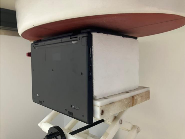
Testing Setup for Body, Back of Display Screen at 0 mm
