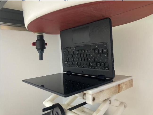
Testing Setup for Body, Front Side of Laptop at 0 mm
