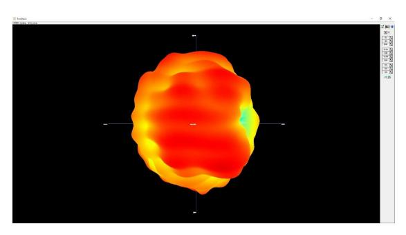
Max Antenna 3D Radiation Pattern 5150-5250 MHz
