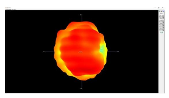
Max Antenna 3D Radiation Pattern 5150-5250 MHz
