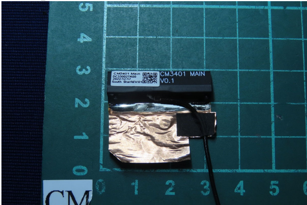
(40) EUT Photo_South Star Main Antenna
