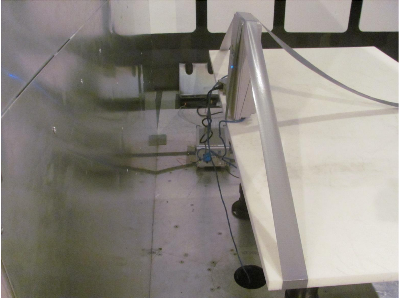
Photograph 3.2-2: Conducted emissions setup
