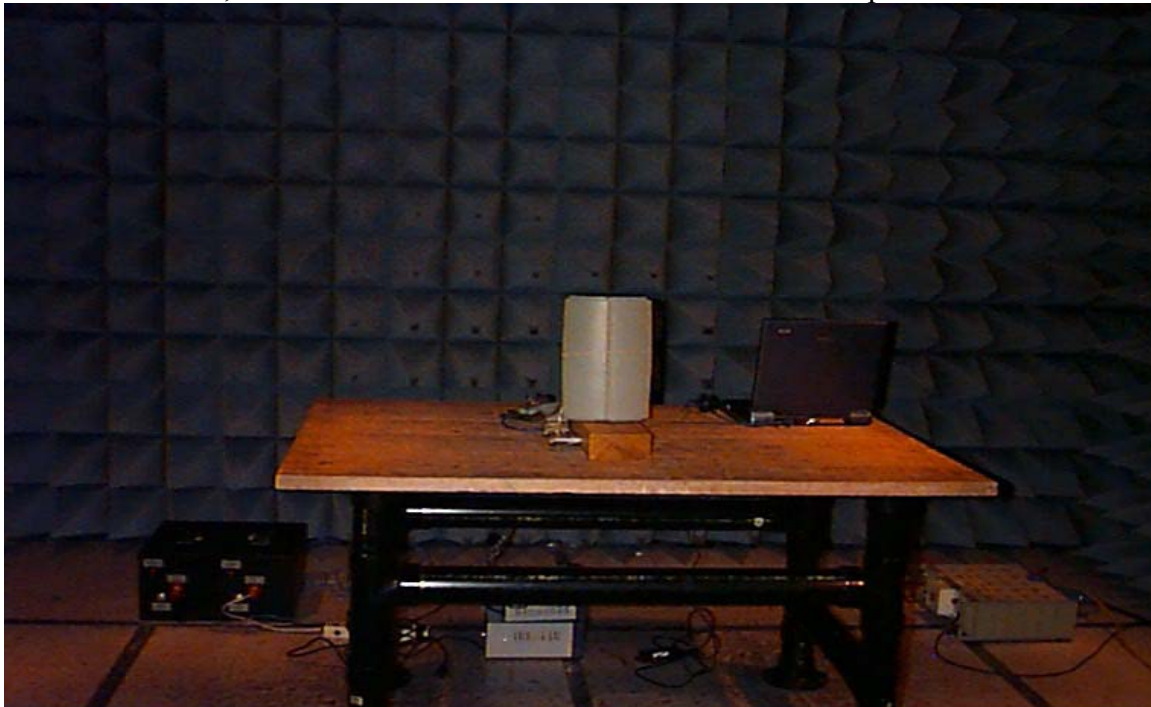
BelAir Networks, 5GHz U-NII Band Module Emissions Test Set Up
