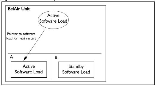
Under normal operating conditions, the contents of the two software load banks are identical. During a software upgrade, the new software load is copied into the standby bank at the time of the upgrade.
