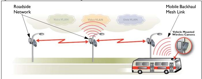
A BelAir20E with mobile backhaul mesh links can support uninterrupted high-performance broadband connectivity for critical applications, including voice and video, as the vehicle moves throughout the wireless mesh at speeds up to 150 mph (240 kph).
