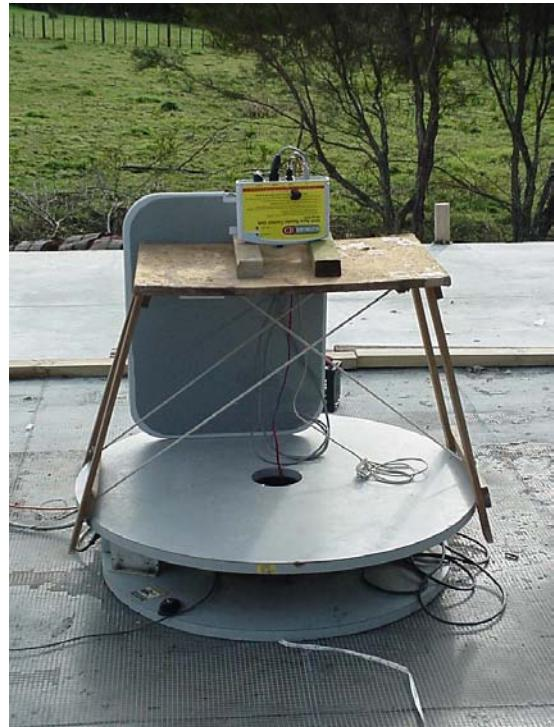
**Radiated Emissions Test Set Up – Two antennas**
