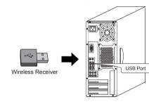
2. Your computer's operating system will automatically detect and connect the device (this device is plug and play, no driver is required). Your wireless device is now ready to use.
