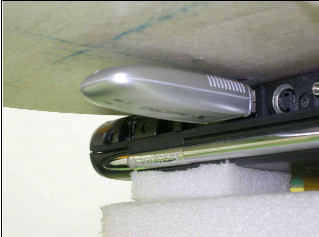
The bottom of the EUT to the flat phantom distance 6 mm
