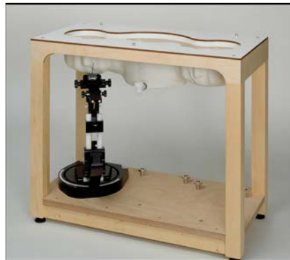
Picture C.10: SAM Twin Phantom
