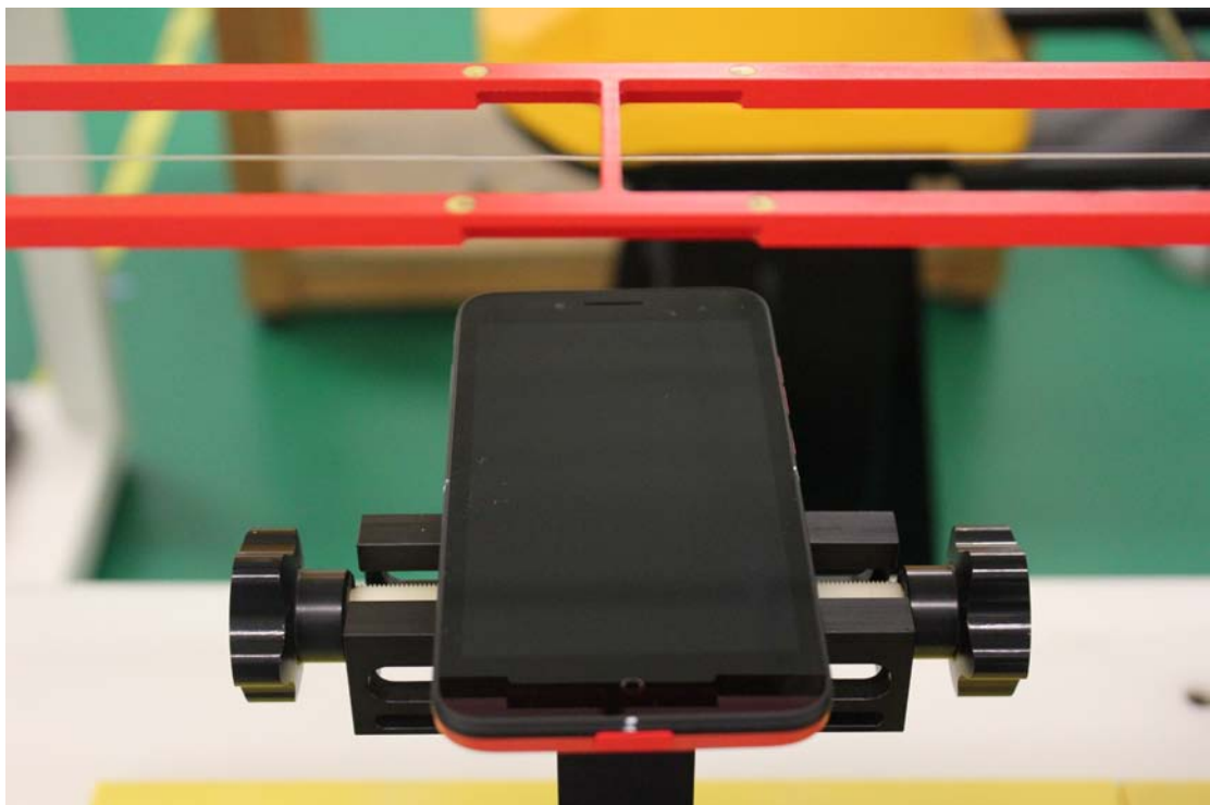
Picture 2: EUT Positioning for RF/T-coil
