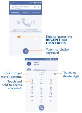
Enter the desired number from the keyboard directly or select a contact from CONTACTS or RECENT by sliding or touching tabs, then choose your target SIM card and touch on to place the call
