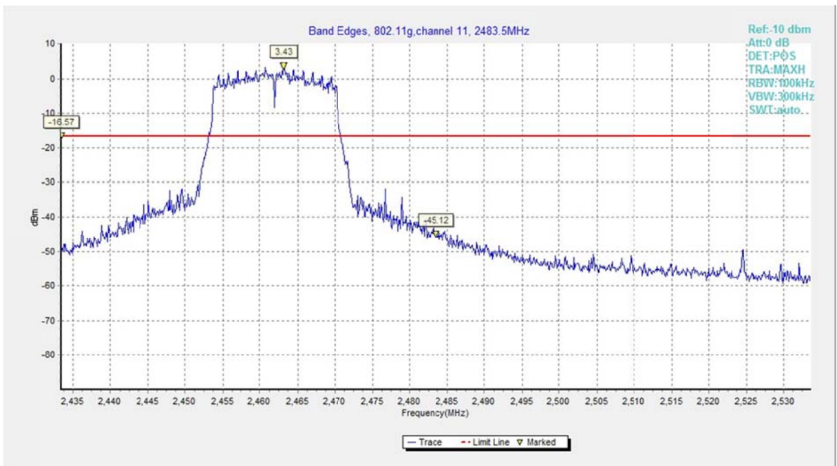
Fig.A.5.4 Band Edges (802.11g, Ch 11)
