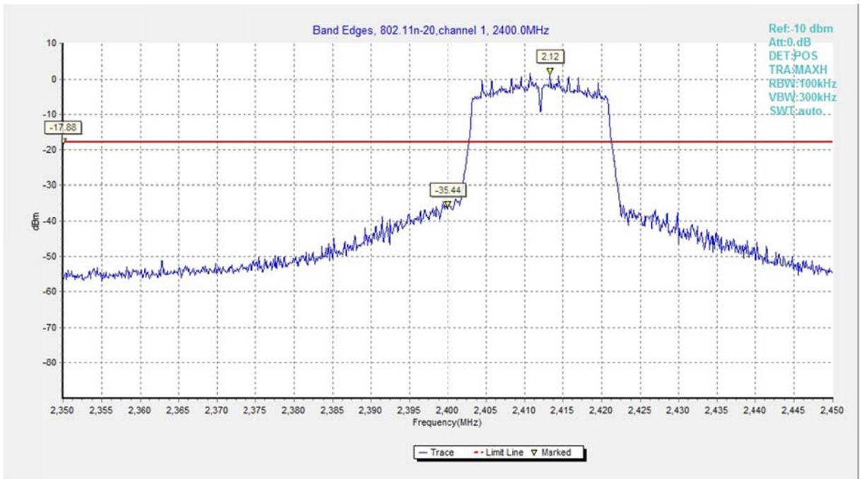
Fig.A.5.5 Band Edges (802.11n-HT20, Ch 1)
