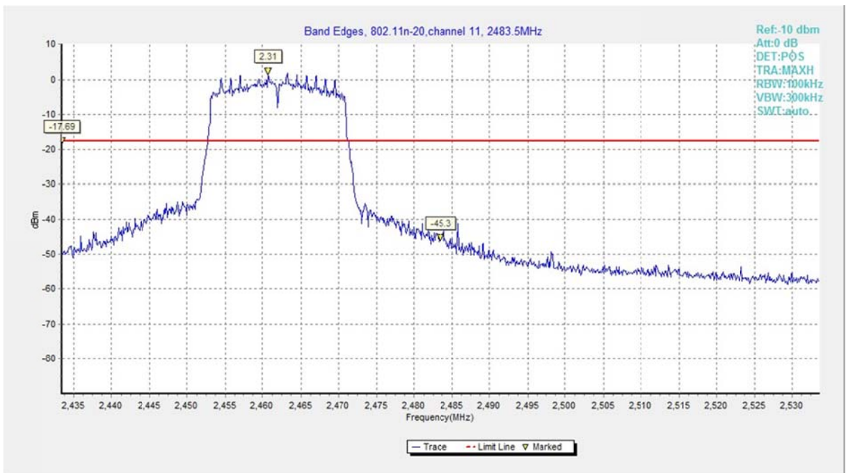
Fig.A.5.6 Band Edges (802.11n-HT20, Ch 11)
