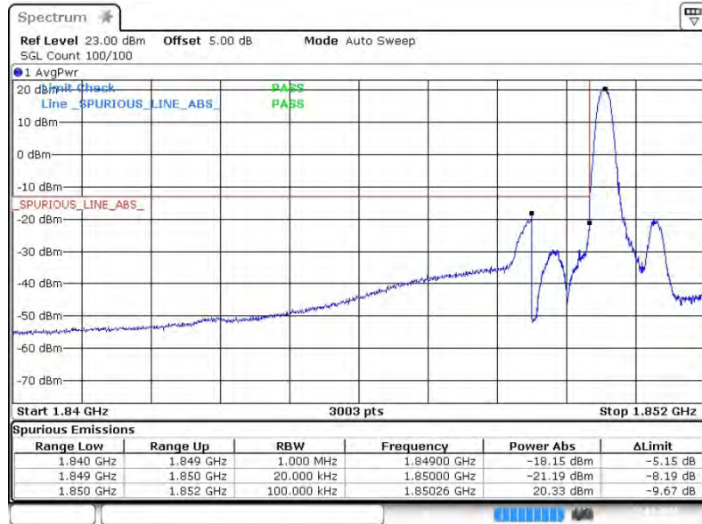
Lower Band Edge Plot for QPSK-RB Size 1, RB Offset 0
