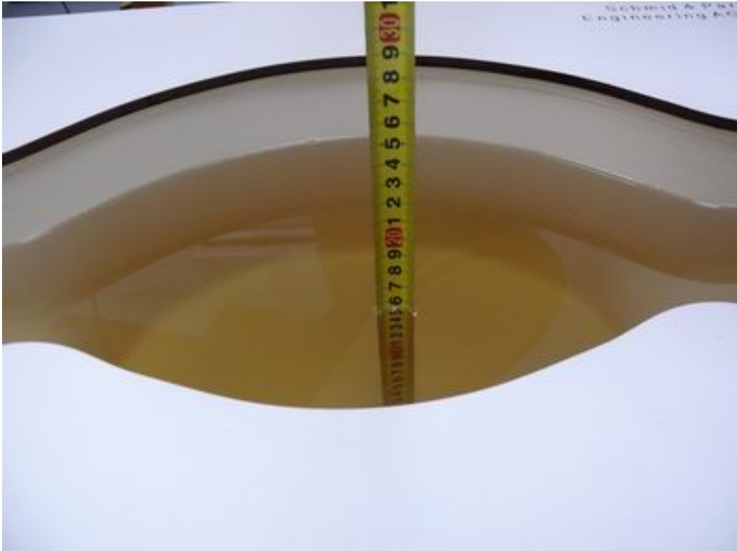
Picture 1: Liquid depth in the flat Phantom (835MHz, 15.4cm depth)
