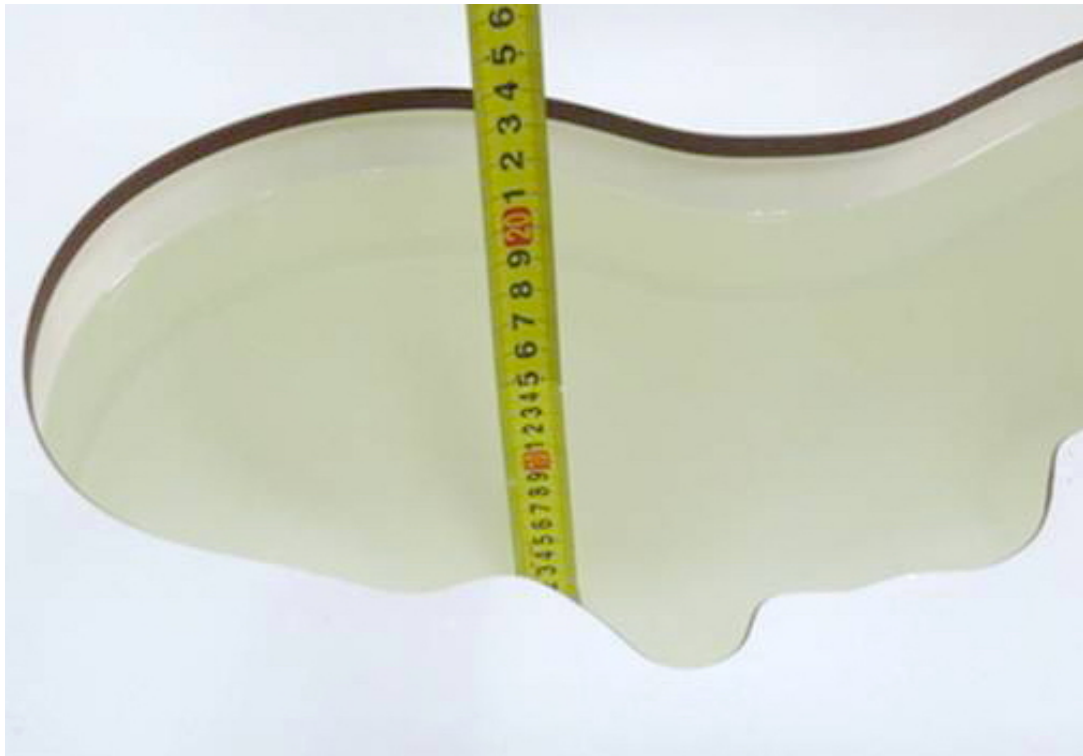
Picture 10: Liquid depth in the head Phantom (2600 MHz, 15.4cm depth)
