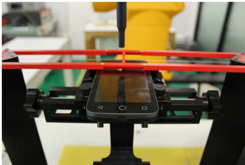
Picture 2: EUT Positioning for RF
