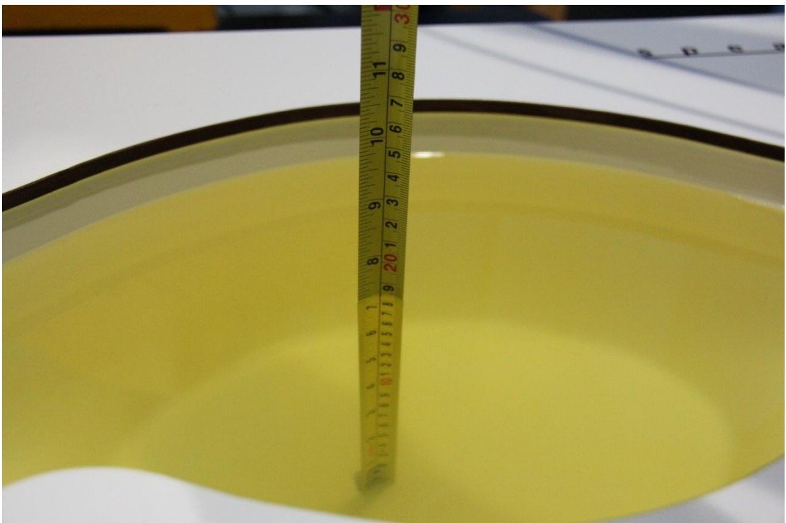
Picture 7-6 Liquid depth in the Flat Phantom (1900MHz)
