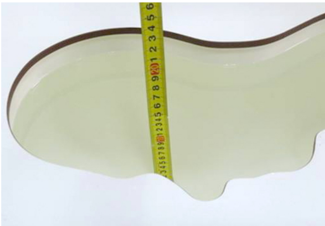
Picture 11: Liquid depth in the head Phantom (2450 MHz, 15.4cm depth)
