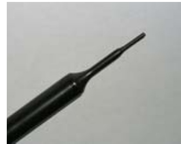
Picture C.2 Near-field Probe
