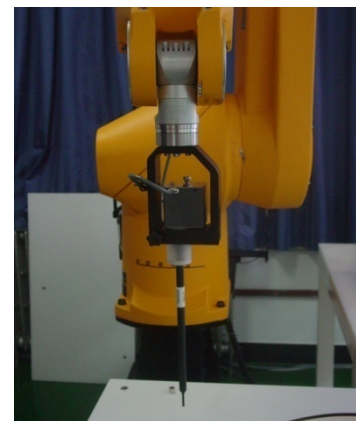
Picture C.3 E-field Probe
