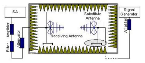
In the chamber, a substitution antenna for the frequency band of interest is placed at the reference point of the chamber. An RF signal source for the frequency band of interest is connected to the substitution antenna with a cable that has been constructed to not interfere with the radiation pattern of the antenna. A power ( $P_{Mea}$ ) is applied to the input of the substitution antenna. Adjust the level of the signal generator output until the value of the
