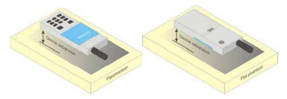
Picture D.4 Test positions for body-worn devices
