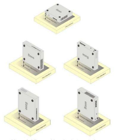
Picture D.5 Test positions for desktop devices
