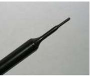
Picture C.2 Near-field Probe
