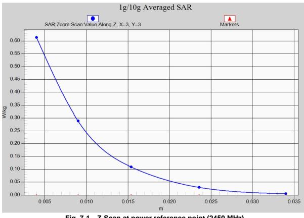
Fig. 7-1 Z-Scan at power reference point (2450 MHz)
