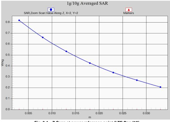
Fig. 6-1 Z-Scan at power reference point (LTE Band13)
