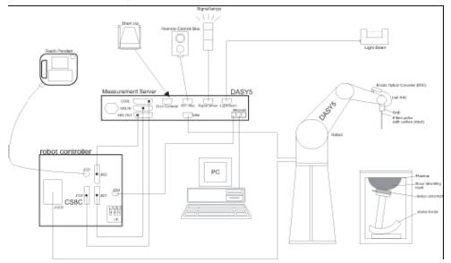
Picture C.1 SAR Lab Test Measurement Set-up
