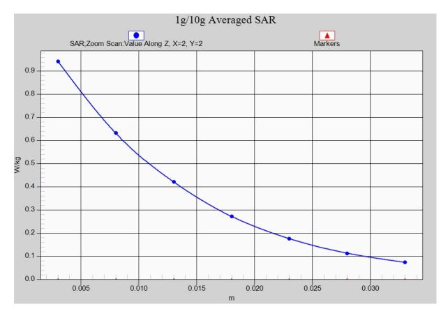
Fig.4-1 Z-Scan at power reference point (CDMA BC1)
