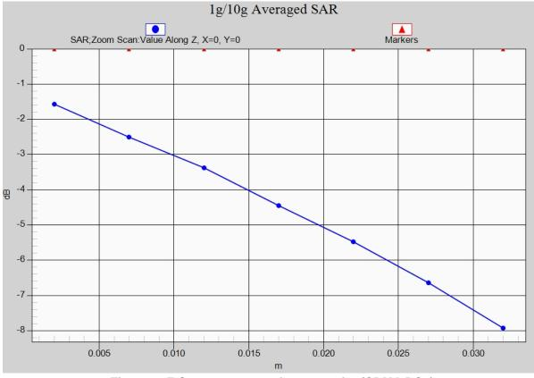
Fig. 1-1 Z-Scan at power reference point (CDMA BC0)
