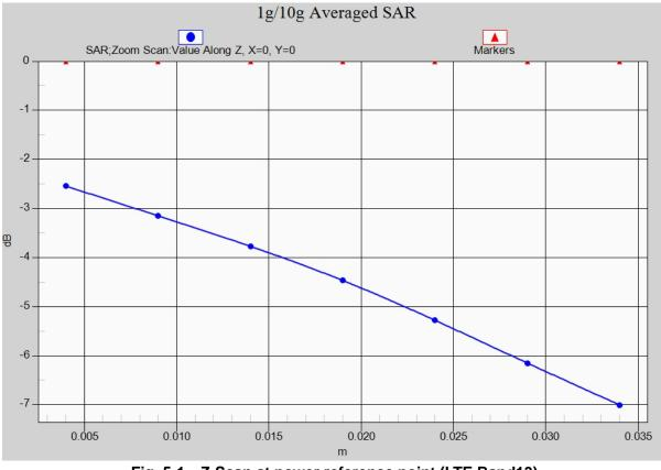
Fig. 5-1 Z-Scan at power reference point (LTE Band13)
