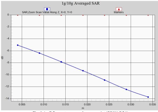
Fig. 3-1 Z-Scan at power reference point (CDMA BC1)
