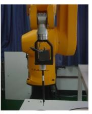
**Picture C.3 E-field Probe**
