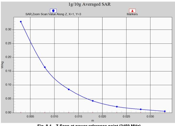
Fig. 8-1 Z-Scan at power reference point (2450 MHz)
