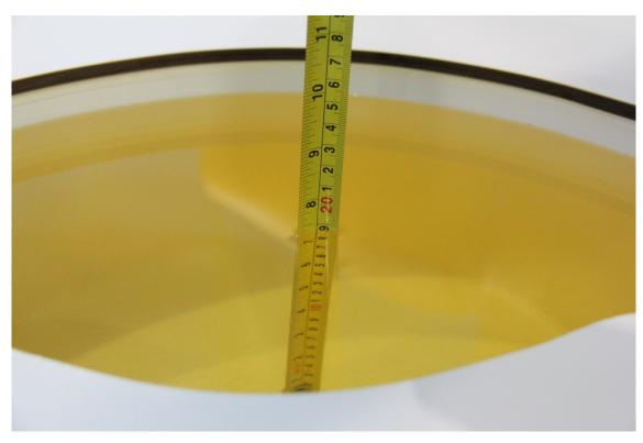
Picture 7-4: Liquid depth in the Flat Phantom (835 MHz)
