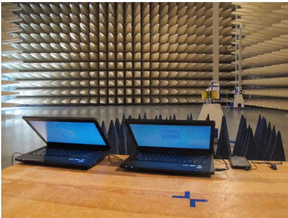
Radiated Emissions Test Setup
