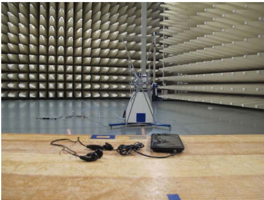
Spurious Radiated Emissions Test setup (30MHz~1GHz)
