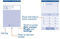
Enter the desired number from the keyboard directly or select a contact from **Contacts** or **Call log** by sliding or touching tabs, then touch  $\checkmark$  to place the call.
