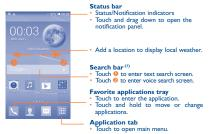
Home screen is provided in an extended format to allow more space for adding applications, shortcuts etc. Slide the Home screen horizontally left and right to get a complete view of the Home screen. The row of small squares at the lower part of the screen indicates which screen you are viewing.
