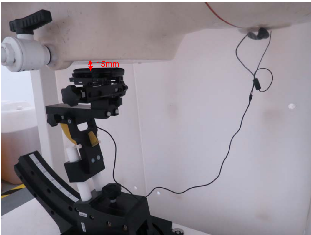
Picture 14: Back Side with earphone, the distance from handset to the bottom of the Phantom is 15mm(Fold closed)
