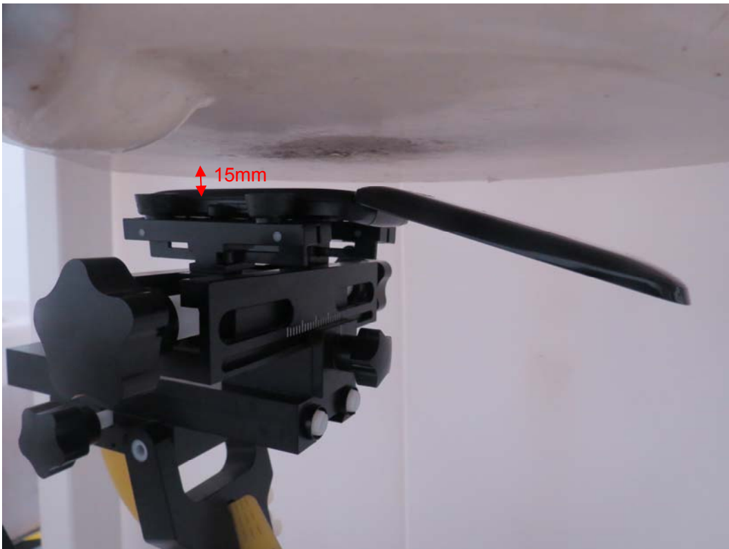
Picture 13: Back Side, the distance from handset to the bottom of the Phantom is 15mm (Fold open)
