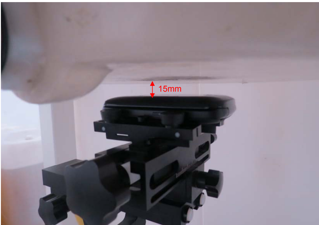
Picture 12: Front Side, the distance from handset to the bottom of the Phantom is 15mm (Fold closed)
