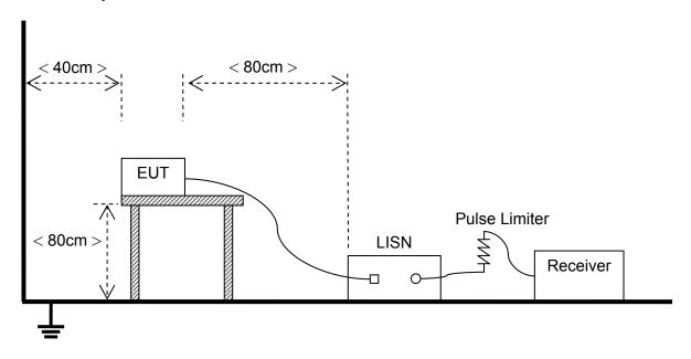
The EUT is placed on a 0.8m high insulating table, which stands on the grounded conducting floor, and keeps 0.4m away from the grounded conducting wall. The EUT is connected to the power mains through a LISN which provides  $50\Omega/50\mu H$  of coupling impedance for the measuring instrument. A Pulse Limiter is used to protect the measuring instrument. The factors of the whole test system are calibrated to correct the reading.
