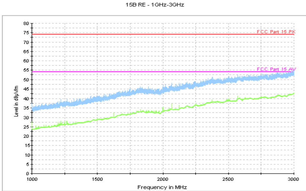
Figure A.5 Radiated Emission from 1GHz to 3GHz
