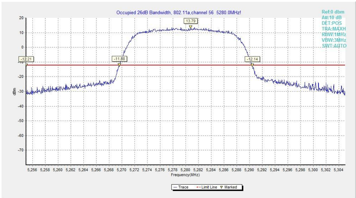
Fig. 5 Occupied 26dB Bandwidth (802.11a, 5280MHz)
