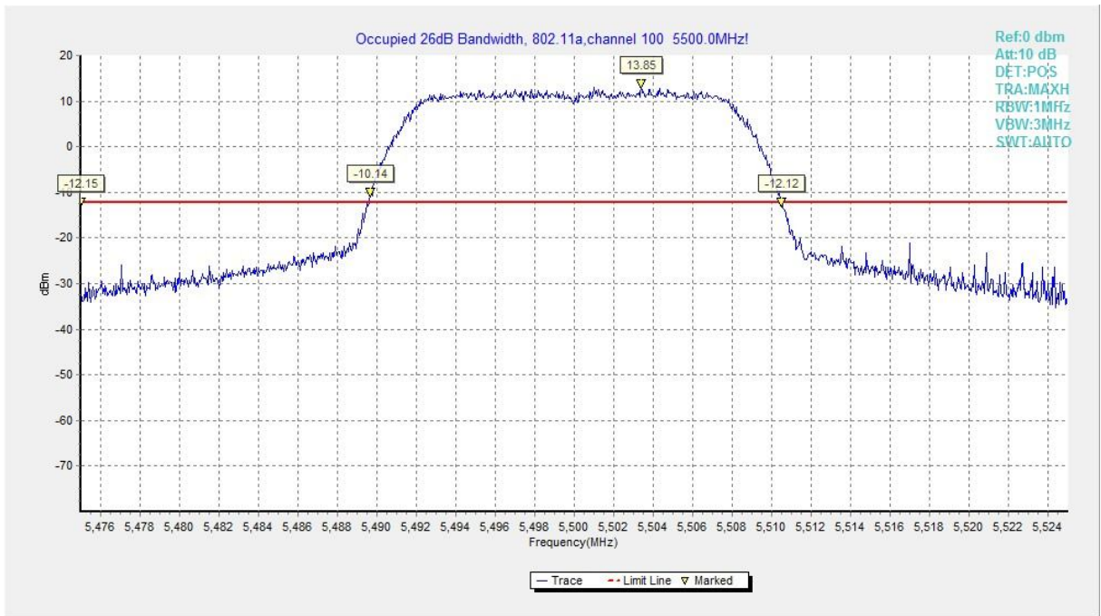
Fig. 7 Occupied 26dB Bandwidth (802.11a, 5500MHz)
