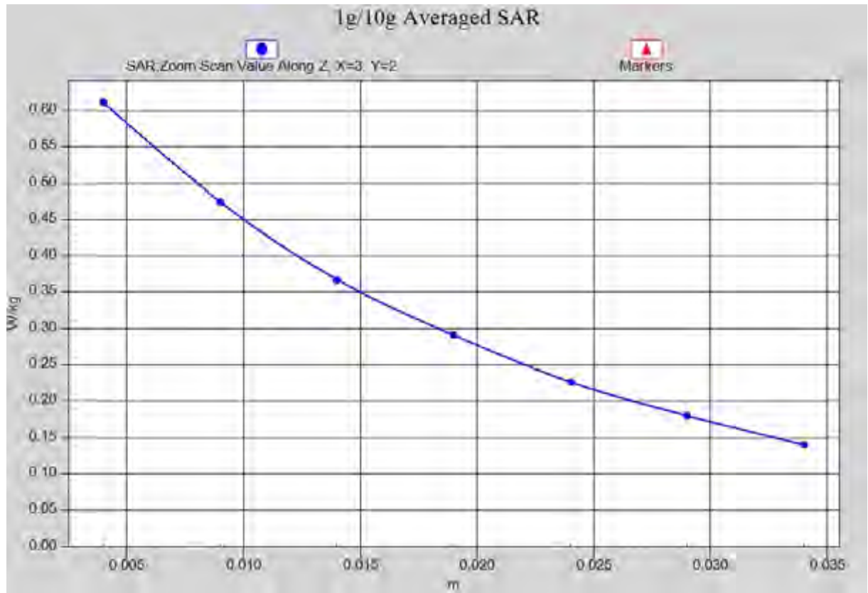
Fig. 1-1 Z-Scan at power reference point (850 MHz CH251)
