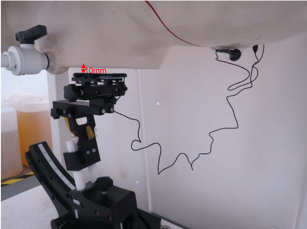
Picture 25: Back Side with Earphone, the distance from handset to the bottom of the Phantom is 10mm
