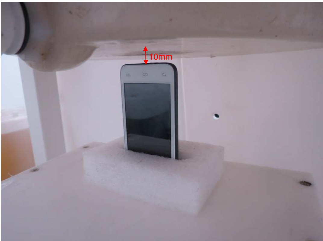
Picture 24: Bottom Edge, the distance from handset to the bottom of the Phantom is 10mm
