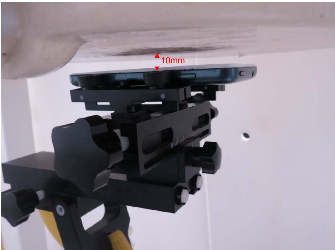
Picture 20: Front Side, the distance from handset to the bottom of the Phantom is 10mm
