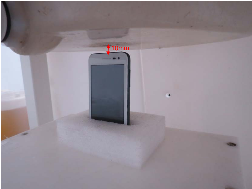
Picture 23: Top Edge, the distance from handset to the bottom of the Phantom is 10mm
