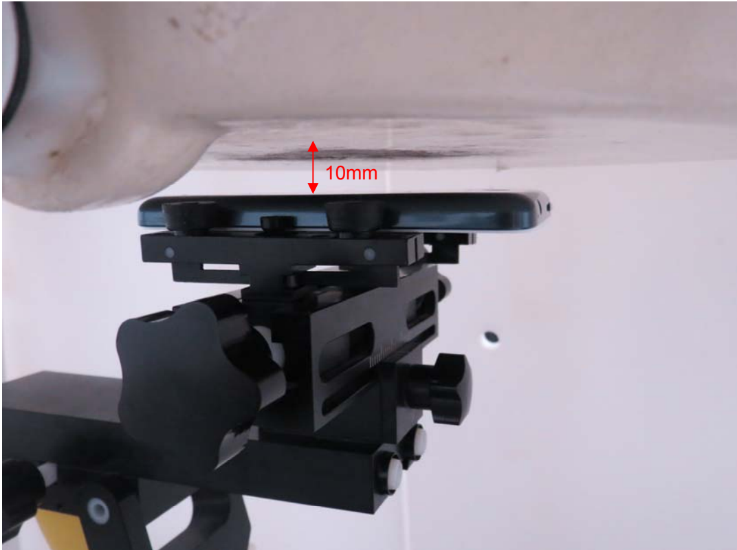
Picture 19: Back Side, the distance from handset to the bottom of the Phantom is 10mm
