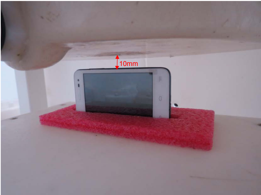
Picture 22: Right Edge, the distance from handset to the bottom of the Phantom is 10mm
