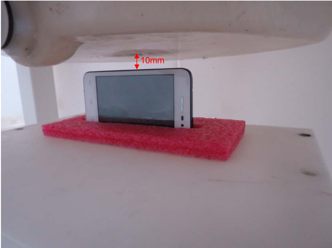
Picture 21: Left Edge, the distance from handset to the bottom of the Phantom is 10mm
