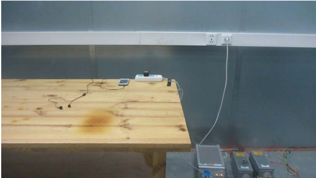
Picture 3 Conducted Emission Test Setup
