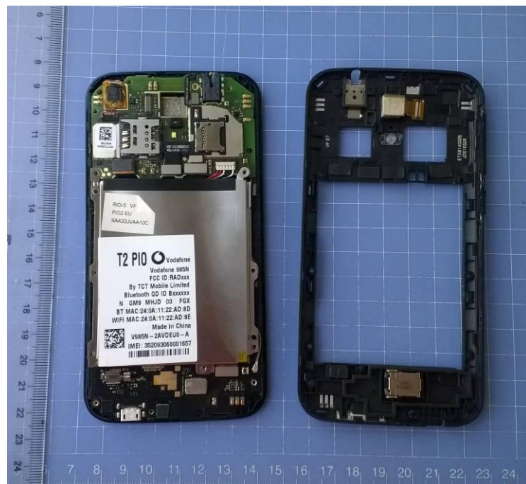
Pic A-4 Mobile phone Disassembly
