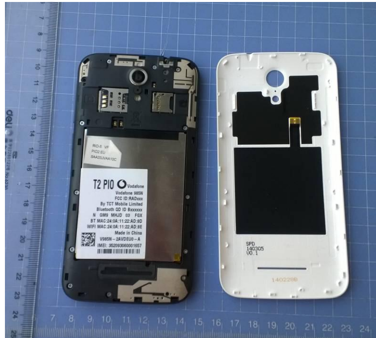
Pic A-3 Mobile phone Disassembly
