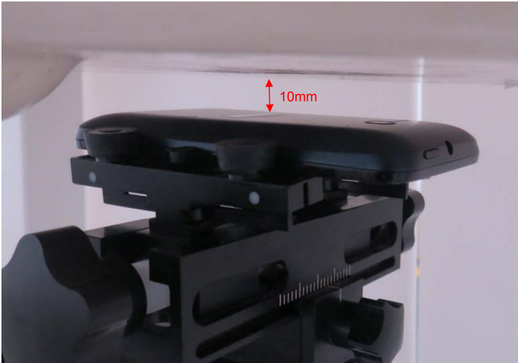
Picture 15: Back Side, the distance from handset to the bottom of the Phantom is 10mm
