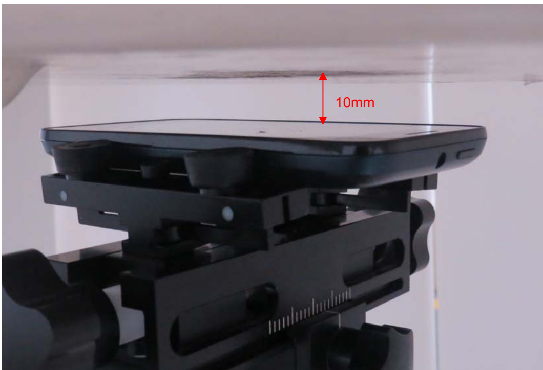
Picture 16: Front Side, the distance from handset to the bottom of the Phantom is 10mm
