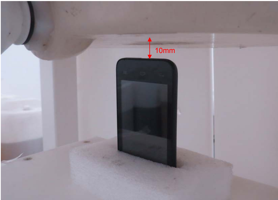
Picture 20: Bottom Edge, the distance from handset to the bottom of the Phantom is 10mm
