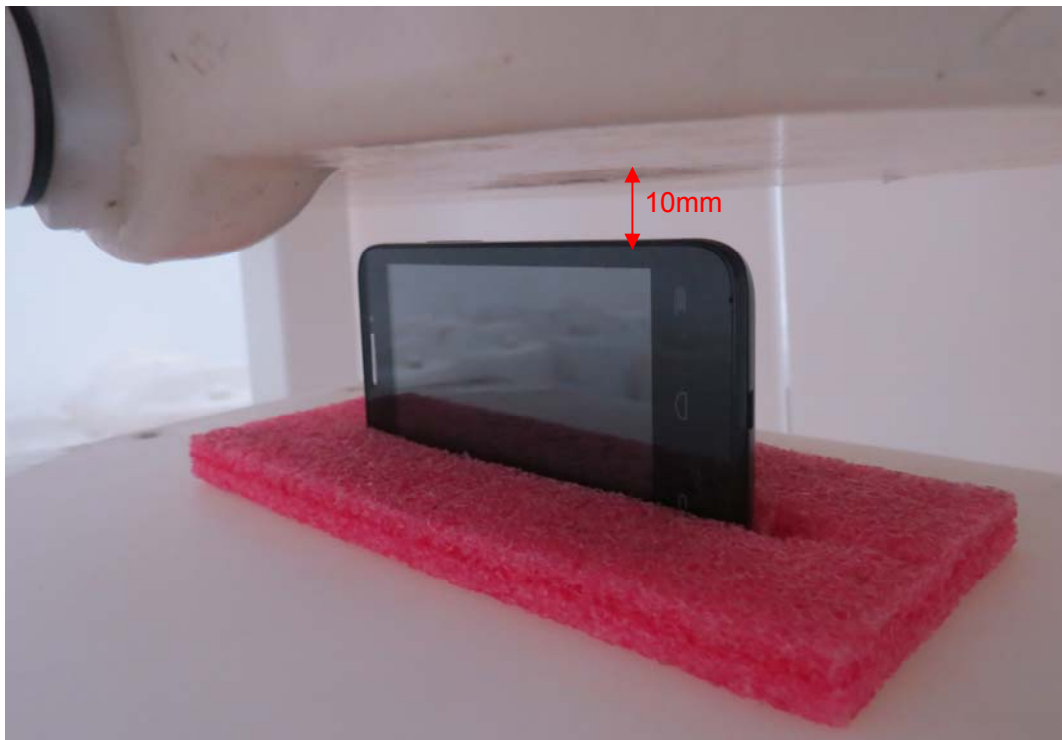
Picture 18: Right Edge, the distance from handset to the bottom of the Phantom is 10mm
