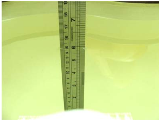
Fig 6.1 Photo of Liquid Height for Head SAR
