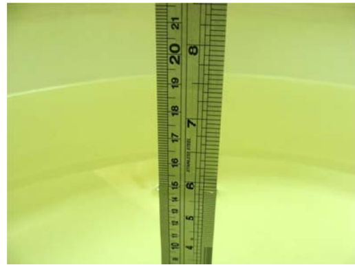
Fig 6.2 Photo of Liquid Height for Body SAR
