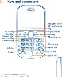
Navigation key Press to go left/right/up/down Press to access function
