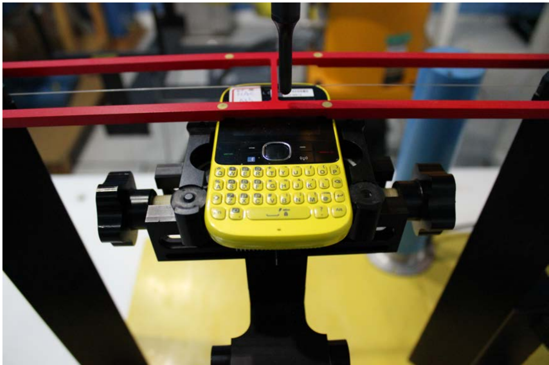
Picture 2: EUT Positioning for RF
