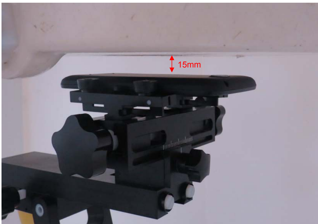
Picture 20: Front Side, the distance from handset to the bottom of the Phantom is 15mm (A564C)
