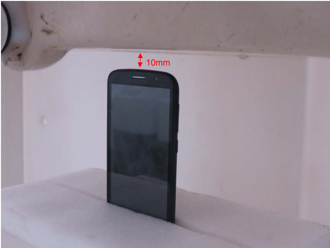
Picture 17: Top Edge, the distance from handset to the bottom of the Phantom is 10mm(A564R)
