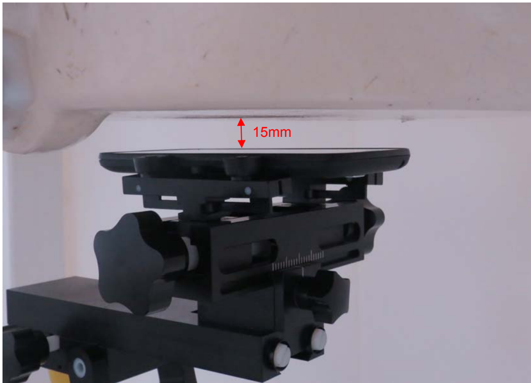
Picture 19: Back Side, the distance from handset to the bottom of the Phantom is 15mm (A564C)
