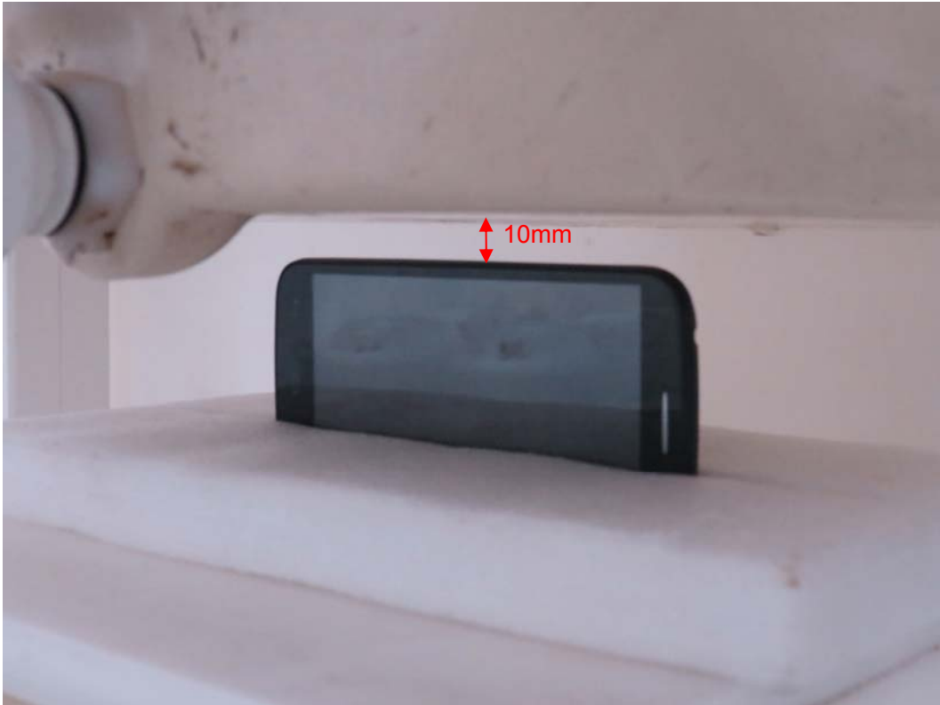
Picture 15: Left Edge, the distance from handset to the bottom of the Phantom is 10mm(A564R)
