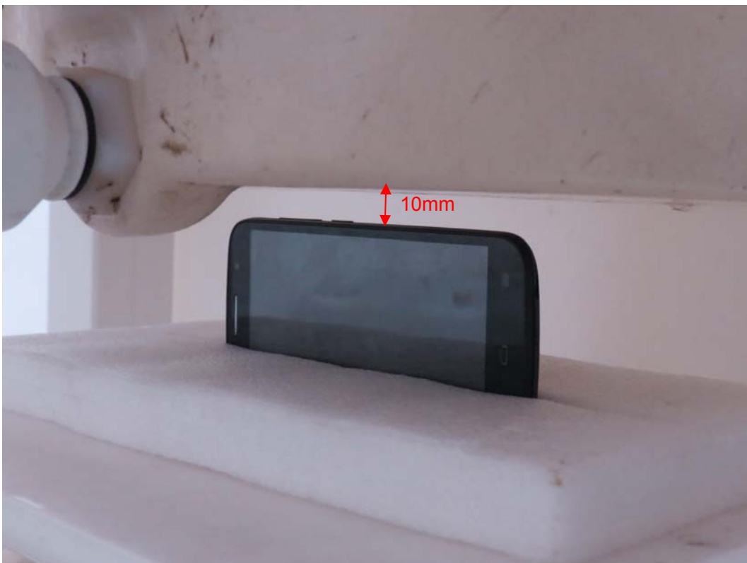
Picture 16: Right Edge, the distance from handset to the bottom of the Phantom is 10mm(A564R)
