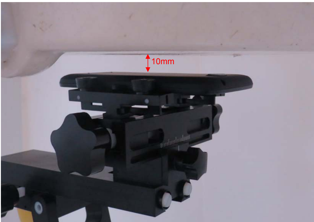
Picture 14: Front Side, the distance from handset to the bottom of the Phantom is 10mm(A564R)
