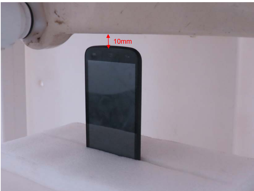
Picture 18: Bottom Edge, the distance from handset to the bottom of the Phantom is 10mm(A564R)
