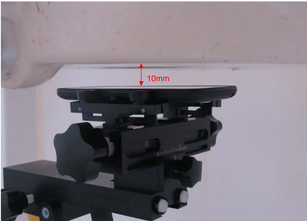
Picture 13: Back Side, the distance from handset to the bottom of the Phantom is 10mm(A564R)
