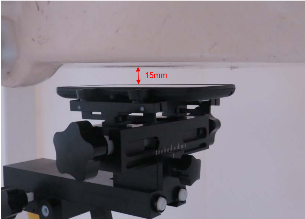
Picture 13: Back Side, the distance from handset to the bottom of the Phantom is 15mm (A564C)
