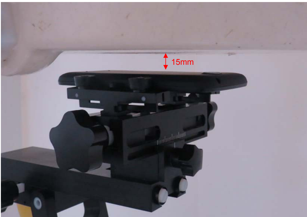
Picture 14: Front Side, the distance from handset to the bottom of the Phantom is 15mm (A564C)
