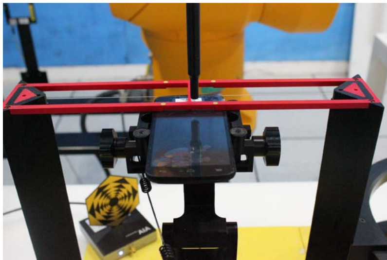
Picture 2: EUT Positioning for RF
