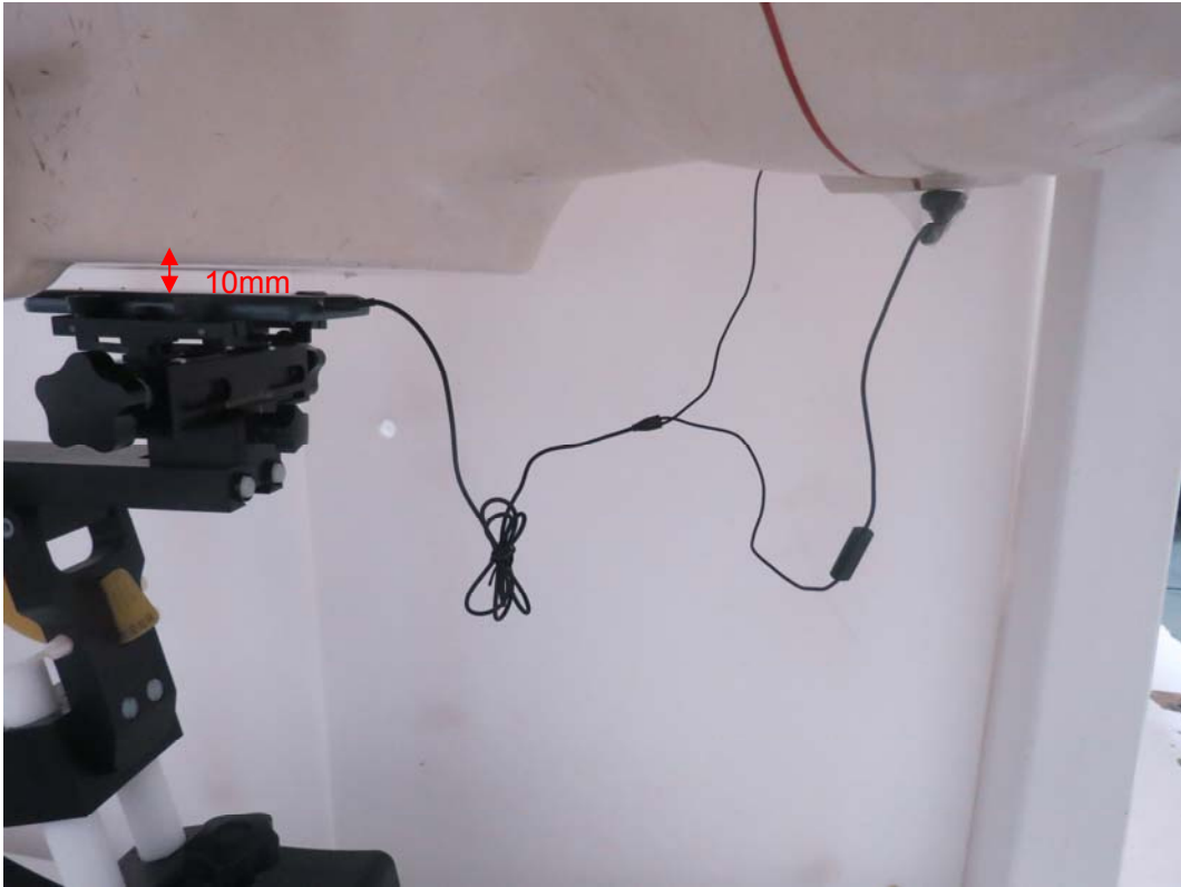
Picture 23: Back Side with earphone, the distance from handset to the bottom of the Phantom is 15mm
