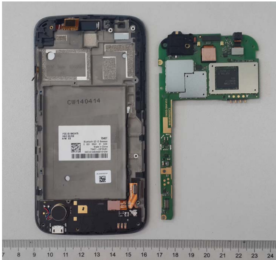
Mobile Phone Disassembly
