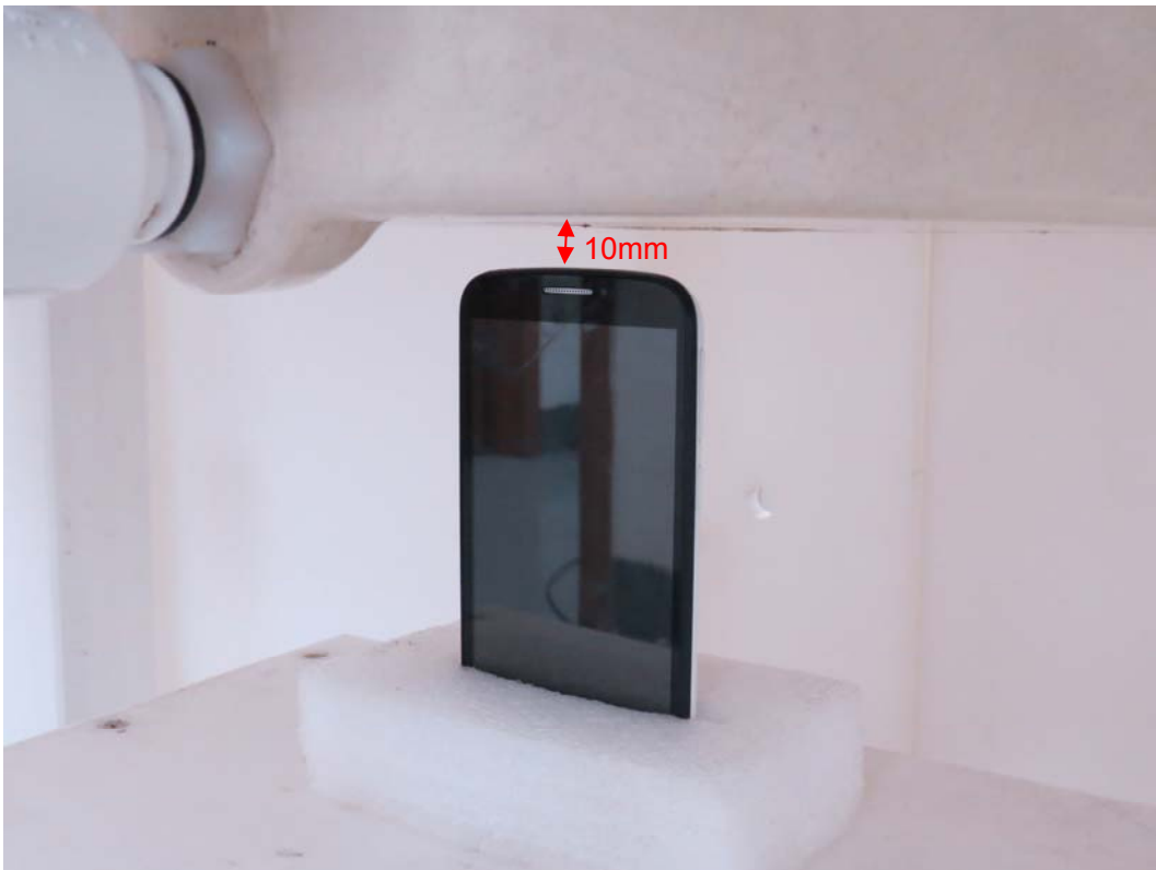
Picture 17: Top Edge, the distance from handset to the bottom of the Phantom is 10mm
