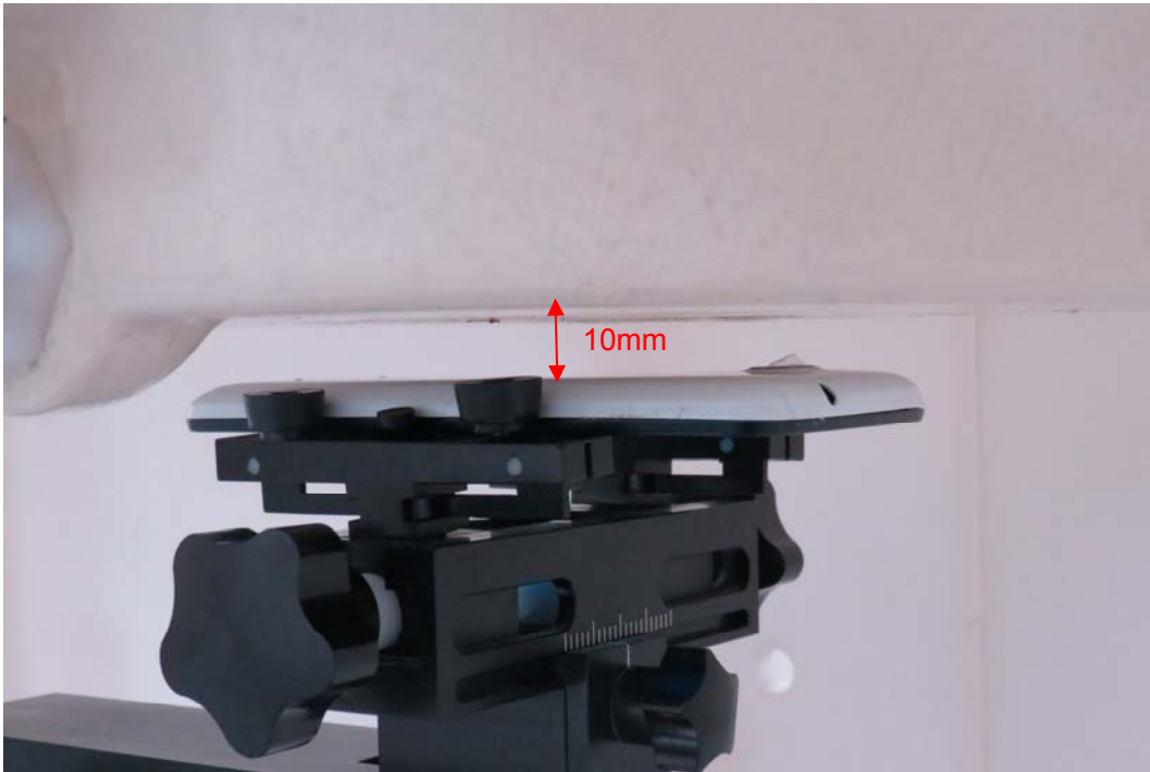
Picture 13: Back Side, the distance from handset to the bottom of the Phantom is 10mm
