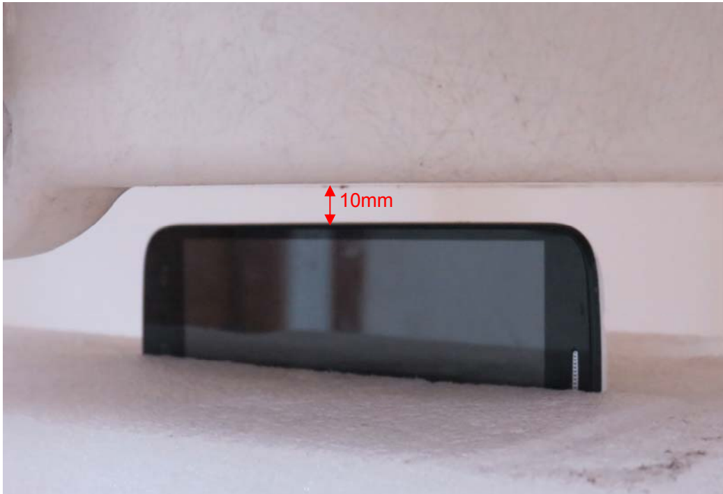
Picture 15: Left Edge, the distance from handset to the bottom of the Phantom is 10mm
