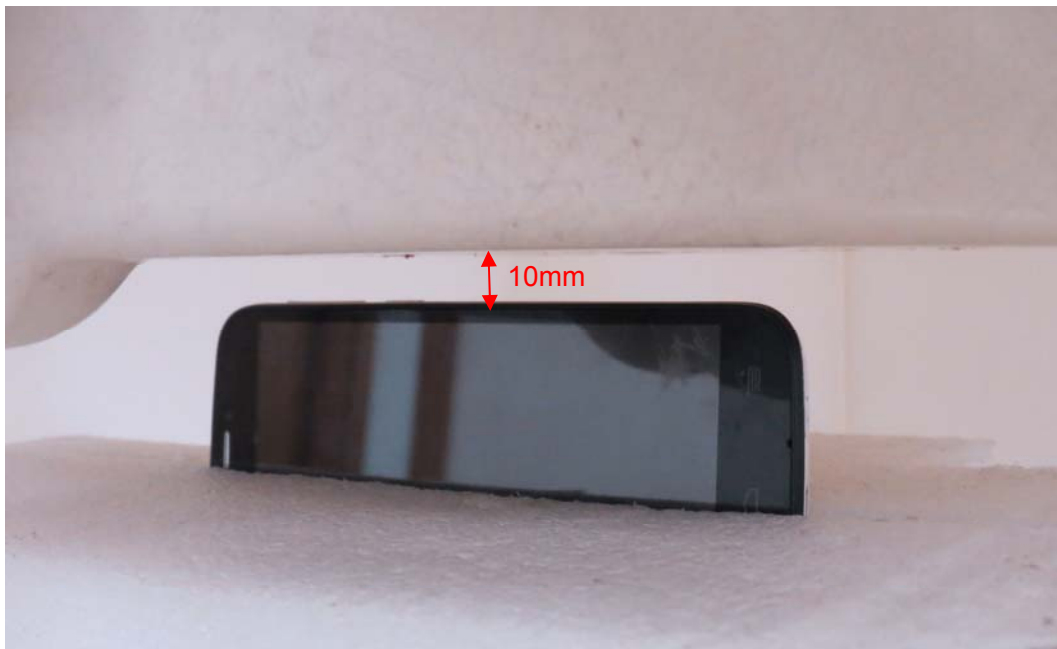
Picture 16: Right Edge, the distance from handset to the bottom of the Phantom is 10mm
