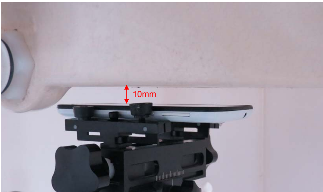
Picture 14: Front Side, the distance from handset to the bottom of the Phantom is 10mm
