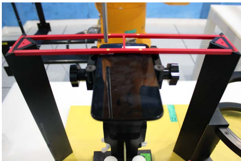
Picture 3: EUT Positioning for T-coil
