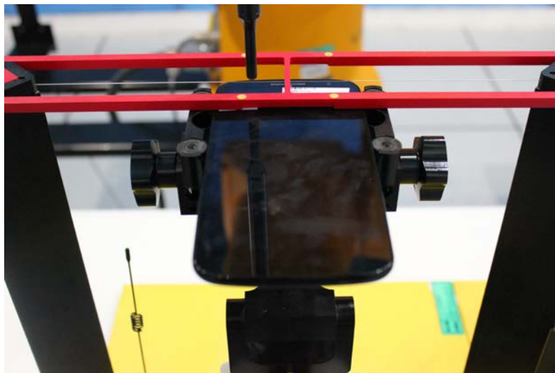
Picture 2: EUT Positioning for RF
