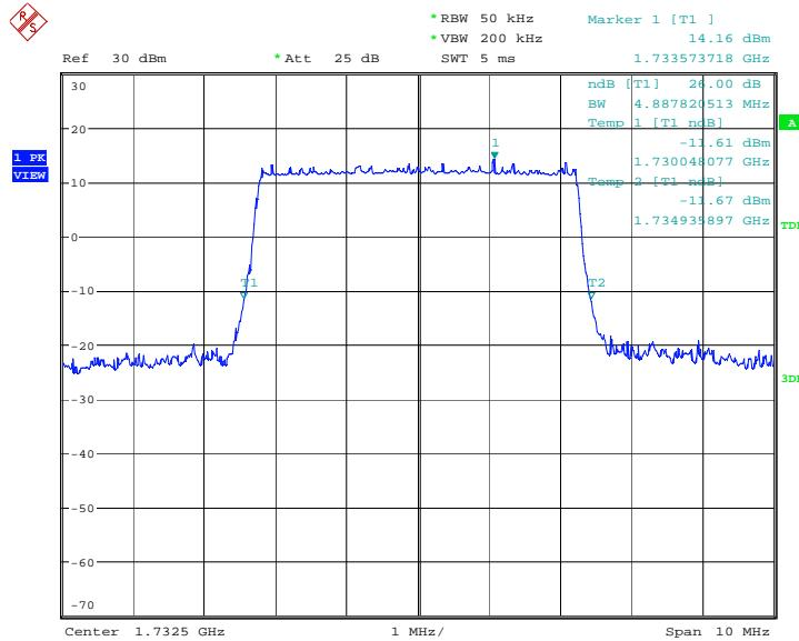
**LTE band 4, 5MHz Bandwidth,16QAM (-26dBc BW)**
